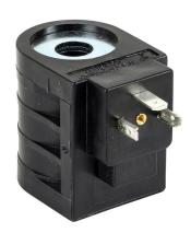
Bucher solenoid coil, replacement, 120 VAC, 22W, DIN 43650 connector. For use with Bucher solenoid valve 51020850999.
