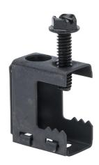
Minerallac screw-on beam clamp, 100 lbs. Package of 100. For use with flanges up to 1/2in and up to 3/8 threaded rod with nut (nut not included).
