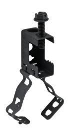
Minerallac screw-on beam clamp conduit hanger assembly, spring clip, bottom mount, 100 lbs. Package of 100. For use with flanges up to 1/2in and 1/2 or 3/4in conduit.
