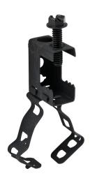
Minerallac screw-on beam clamp conduit hanger assembly, spring clip, bottom mount, 100 lbs. Package of 10. For use with flanges up to 1/2in and 1/2 or 3/4in conduit.
