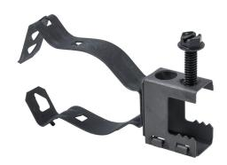
Minerallac screw-on beam clamp conduit hanger assembly, spring clip, back mount, 100 lbs. Package of 10. For use with flanges up to 1/2in and 1-1/2in conduit.
