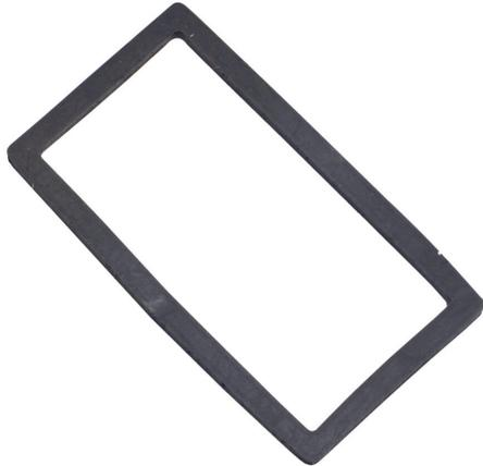
Trumeter gasket, nitrile rubber, NEMA 4/4X. For use with Trumeter 6300 and 6320 type rectangular DIN 1/32 counters and hour meters.
