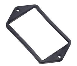
Trumeter gasket, neoprene, NEMA 4/4X. For use with Trumeter 722, 732, 3400 and 3410 type rectangular 2-hole counters and hour meters.
