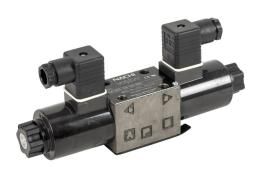
Bucher solenoid valve, D03, 4-port (4-way), 3-position, center float, double solenoid, cast iron body, momentary manual override, Cv=21.1, 24 VDC.
