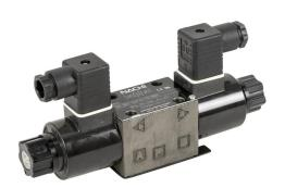
Bucher solenoid valve, D03, 4-port (4-way), 3-position, center open, double solenoid, cast iron body, momentary manual override, Cv=13.2, 120 VAC.
