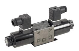
Bucher solenoid valve, D03, 4-port (4-way), 3-position, center tandem, double solenoid, cast iron body, momentary manual override, Cv=13.2, 24 VDC.
