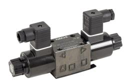
Bucher solenoid valve, D03, 4-port (4-way), 3-position, center tandem, double solenoid, cast iron body, momentary manual override, Cv=13.2, 120 VAC.
