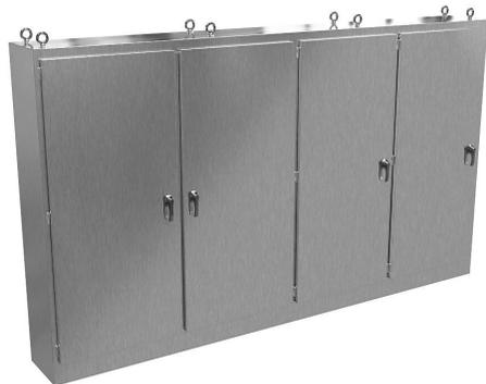
Hammond disconnect enclosure, NEMA 3R/4/4X/12/13, right flange, 90 x 157 x 18in (HxWxD), freestanding, 304 stainless steel, #4 brush finish, 4-door, 3-point padlocking handle.
