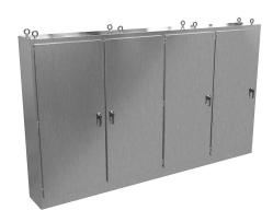
Hammond disconnect enclosure, NEMA 3R/4/4X/12/13, right flange, 90 x 157 x 18in (HxWxD), freestanding, 304 stainless steel, #4 brush finish, 4-door, 3-point padlocking handle.
