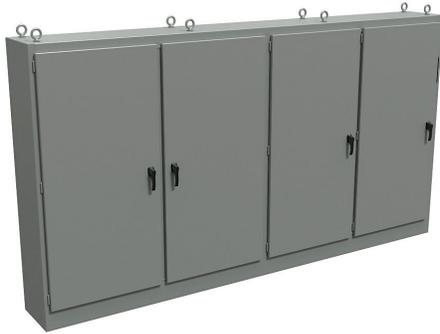
Hammond disconnect enclosure, NEMA 12, right flange, 84 x 157 x 18in (HxWxD), freestanding, carbon steel, ANSI 61 gray, powder coat finish, 4-door, 3-point padlocking handle.
