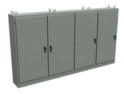
Hammond disconnect enclosure, NEMA 12, right flange, 84 x 157 x 18in (HxWxD), freestanding, carbon steel, ANSI 61 gray, powder coat finish, 4-door, 3-point padlocking handle.
