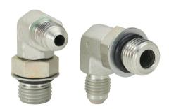
HY-TECH hydraulic fluid adapter, elbow, plated steel body, (1) -4 male JIC 37 deg and (1) -6 male o-ring boss. Package of 2.
