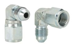
HY-TECH hydraulic fluid adapter, elbow, plated steel body, (1) -4 male JIC 37 deg and (1) -4 female JIC 37 deg. Package of 2.
