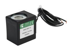
Spartan solenoid coil, 220 VAC, 11.5 VA, 18mm DIN style wiring plug. For use with 6100, 6200 and 6222 series Spartan valves.
