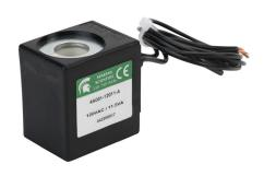
Spartan solenoid coil, 120 VAC, 11.5 VA, 18mm DIN style wiring plug. For use with 6100, 6200 and 6222 series Spartan valves.
