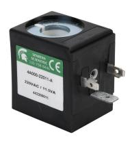
Spartan solenoid coil, 220 VAC, 11.5 VA, 18mm DIN style wiring plug. For use with 6100, 6200 and 6222 series Spartan valves.
