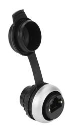
LUTZE Cat5e Ethernet bulkhead connector, RJ45 female 8-wire/8-pin to RJ45 female 8-wire/8-pin, shielded, IP65 (cover closed), IP20 (cable inserted), UL Type 2, 3R, 4, 4X, 12 and 13.
