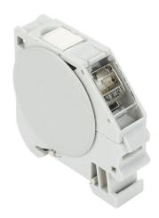
LUTZE Cat6a Ethernet connector, field-wireable, RJ45 female axial 8-wire/8-pin, accepts cable diameter size up to 9mm, 26-22 AWG, TIA-568A color code, insulation displacement (IDC) connection, IP20.
