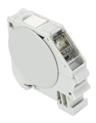
LUTZE Cat6a Ethernet connector, field-wireable, RJ45 female axial 8-wire/8-pin, accepts cable diameter size up to 9mm, 26-22 AWG, TIA-568B color code, insulation displacement (IDC) connection, IP20.
