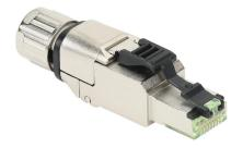
LUTZE Cat6a Ethernet connector, field-wireable, RJ45 male axial 8-wire/8-pin, accepts cable diameter size 5.5-10mm, 26-22 AWG, TIA-568B color code, insulation displacement (IDC) connection, IP20.
