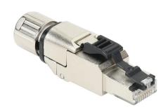
LUTZE Cat6a Ethernet connector, field-wireable, RJ45 male axial 8-wire/8-pin, accepts cable diameter size 5.5-10mm, 24-22 AWG, TIA-568A color code, insulation displacement (IDC) connection, IP20.
