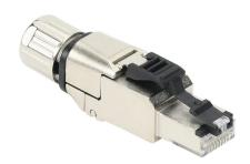
LUTZE Cat6a Ethernet connector, field-wireable, RJ45 male axial 8-wire/8-pin, accepts cable diameter size 5.5-10mm, 24-22 AWG, TIA-568B color code, insulation displacement (IDC) connection, IP20.
