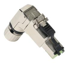
LUTZE Cat6a Ethernet connector, field-wireable, RJ45 male 90-degree 8-wire/8-pin, accepts cable diameter size 5.5-10mm, 26-22 AWG, TIA-568B color code, insulation displacement (IDC) connection, IP20.
