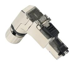
LUTZE Cat6a Ethernet connector, field-wireable, RJ45 male 90-degree 8-wire/8-pin, accepts cable diameter size 5.5-10mm, 24-22 AWG, TIA-568A color code, insulation displacement (IDC) connection, IP20.
