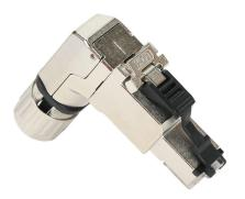
LUTZE Cat6a Ethernet connector, field-wireable, RJ45 male 90-degree 8-wire/8-pin, accepts cable diameter size 5.5-10mm, 24-22 AWG, TIA-568B color code, insulation displacement (IDC) connection, IP20.
