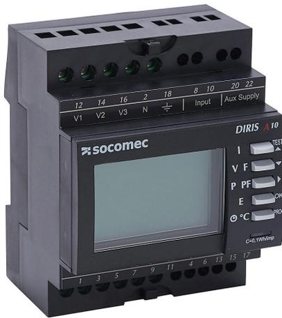
Socomec DIRIS A10 power meter, current and voltage input, 3-line backlit LCD, configurable output, 110-277 VAC operating voltage, Modbus RTU.
