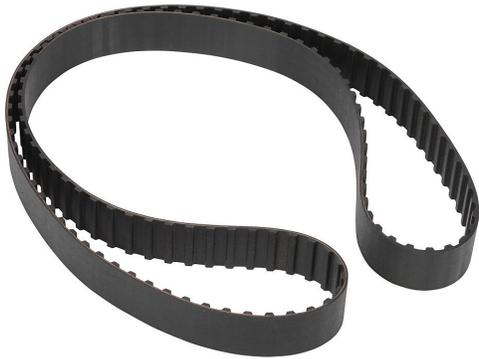
SureMotion timing belt, 3/8in L pitch, 1in wide, 128 tooth, 48in pitch length (circumference), neoprene, fiberglass reinforced.
