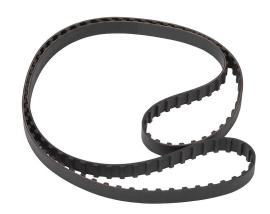
SureMotion timing belt, 3/8in L pitch, 1/2in wide, 128 tooth, 48in pitch length (circumference), neoprene, fiberglass reinforced.
