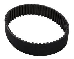
SureMotion timing belt, 8mm 8M pitch, 30mm wide, 60 tooth, 480mm pitch length (circumference), neoprene, fiberglass reinforced.
