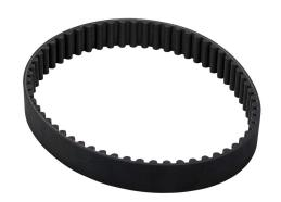
SureMotion timing belt, 8mm 8M pitch, 20mm wide, 60 tooth, 480mm pitch length (circumference), neoprene, fiberglass reinforced.
