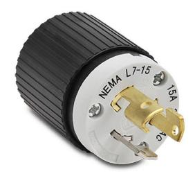
Bryant industrial heavy duty locking blade plug, 15A, 277 VAC, 1-phase, 2-pole, 3-wire, NEMA L7-15, accepts cord size 0.3-0.65in, nylon housing, black and white.
