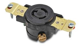
Bryant industrial heavy duty single locking blade receptacle, 15A, 277 VAC, 1-phase, 2-pole, 3-wire, NEMA L7-15, nylon molded housing, black.
