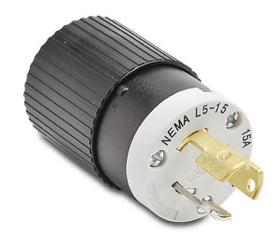
Bryant industrial heavy duty locking blade plug, 15A, 125 VAC, 1-phase, 2-pole, 3-wire, NEMA L5-15, accepts cord size 0.3-0.65in, nylon housing, black and white.
