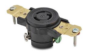
Bryant industrial heavy duty single locking blade receptacle, 15A, 125 VAC, 1-phase, 2-pole, 3-wire, NEMA L5-15, nylon molded housing, black.
