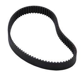
SureMotion timing belt, 5mm 5M pitch, 15mm wide, 93 tooth, 465mm pitch length (circumference), neoprene, fiberglass reinforced.
