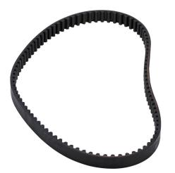
SureMotion timing belt, 5mm 5M pitch, 9mm wide, 93 tooth, 465mm pitch length (circumference), neoprene, fiberglass reinforced.
