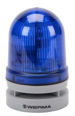
WERMA EvoSIGNAL Midi TwinFLASH series LED audible-visual signal beacon, 110 dB at 1m, (10) selectable tone(s), double flash or EVS (Enhanced Visibility System) flashing (random flashing), blue, 85mm, 115-230 VAC, IP66. Requires mounting adapter.
