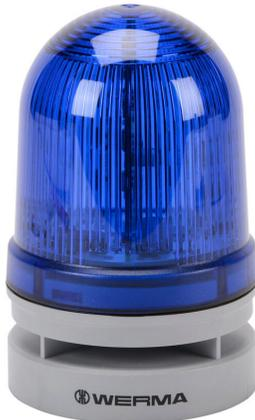
WERMA EvoSIGNAL Midi TwinLIGHT series LED audible-visual signal beacon, 110 dB at 1m, (10) selectable tone(s), permanent or blinking (1 Hz ON for 480ms), blue, 85mm, 12/24 VAC/VDC, IP66. Requires mounting adapter.
