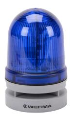
WERMA EvoSIGNAL Midi TwinLIGHT series LED audible-visual signal beacon, 110 dB at 1m, (10) selectable tone(s), permanent or blinking (1 Hz ON for 420ms), blue, 85mm, 115-230 VAC, IP66. Requires mounting adapter.
