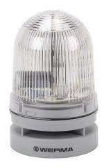
WERMA EvoSIGNAL Midi TwinFLASH series LED audible-visual signal beacon, 110 dB at 1m, (10) selectable tone(s), double flash or EVS (Enhanced Visibility System) flashing (random flashing), clear/white, 85mm, 12/24 VAC/VDC, IP66. Requires mounting adapter.
