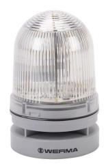
WERMA EvoSIGNAL Midi TwinLIGHT series LED audible-visual signal beacon, 110 dB at 1m, (10) selectable tone(s), permanent or blinking (1 Hz ON for 420ms), clear/white, 85mm, 115-230 VAC, IP66. Requires mounting adapter.
