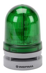
WERMA EvoSIGNAL Midi TwinLIGHT series LED audible-visual signal beacon, 110 dB at 1m, (10) selectable tone(s), permanent or blinking (1 Hz ON for 420ms), green, 85mm, 115-230 VAC, IP66. Requires mounting adapter.
