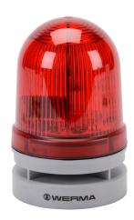
WERMA EvoSIGNAL Midi TwinFLASH series LED audible-visual signal beacon, 110 dB at 1m, (10) selectable tone(s), double flash or EVS (Enhanced Visibility System) flashing (random flashing), red, 85mm, 12/24 VAC/VDC, IP66. Requires mounting adapter.
