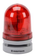
WERMA EvoSIGNAL Midi TwinFLASH series LED audible-visual signal beacon, 110 dB at 1m, (10) selectable tone(s), double flash or EVS (Enhanced Visibility System) flashing (random flashing), red, 85mm, 115-230 VAC, IP66. Requires mounting adapter.
