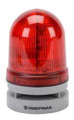
WERMA EvoSIGNAL Midi TwinLIGHT series LED audible-visual signal beacon, 110 dB at 1m, (10) selectable tone(s), permanent or blinking (1 Hz ON for 420ms), red, 85mm, 115-230 VAC, IP66. Requires mounting adapter.
