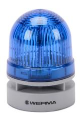
WERMA EvoSIGNAL Mini TwinFLASH series LED audible-visual signal beacon, 95 dB at 1m, continuous/pulse tone(s), double flash or EVS (Enhanced Visibility System) flashing (random flashing), blue, 62mm, 24 VAC/VDC, IP66. Requires mounting adapter.
