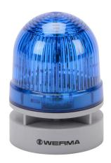
WERMA EvoSIGNAL Mini TwinLIGHT series LED audible-visual signal beacon, 95 dB at 1m, continuous/pulse tone(s), permanent or blinking (1 Hz ON for 410ms), blue, 62mm, 12 VAC/VDC, IP66. Requires mounting adapter.
