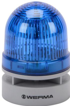
WERMA EvoSIGNAL Mini TwinLIGHT series LED audible-visual signal beacon, 95 dB at 1m, continuous/pulse tone(s), permanent or blinking (1 Hz ON for 420ms), blue, 62mm, 115-230 VAC, IP66. Requires mounting adapter.
